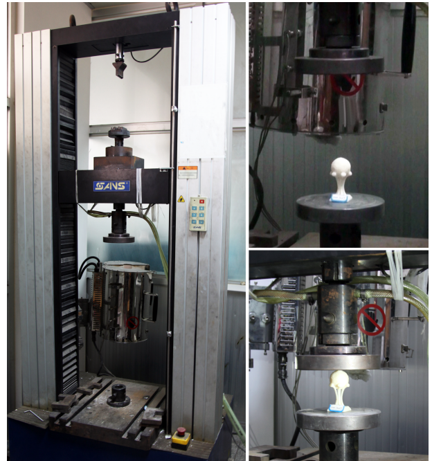
Figure 11: Compression tests using a universal testing machine.
